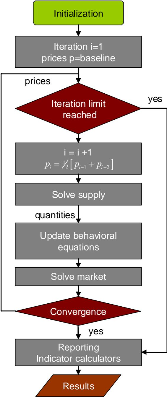
Figure 1: Flowchart of the iterative solution process
