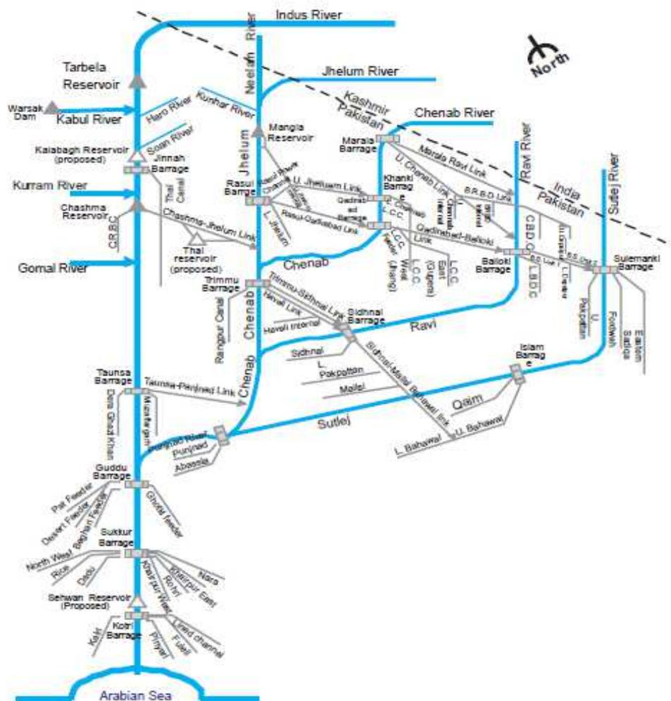
Figure 2 The Indus River basin and irrigation canals (Briscoe & Qamar, 2005b) as modeled in RWSM-Pak
